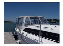
The Bimini Conversion is made up of panels which are zip attached to the stand alone Bimini canvas and the Sprayhood canvas. These panels are measured on the boat to perfection in order to ensure no water penetration and also to make sure compromises are not made to the appearance and the look of the covers on the boat.
