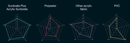
1. Resistant to elongation 2. Breathable fabric 3. Resistant to water 4. Resistant to mold 5. Resistant to breakage caused by age
